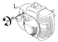
**CAUTION!** If the cutting attachment rotates when the engine is idling the idle adjustment screw T should be turned anti-clockwise until the cutting attachment stops.
